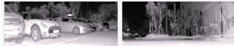
Colorized Image from LiDAR
