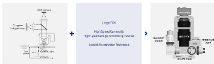
▲ LWSI - Large FOV White light Scanning Interferometer
