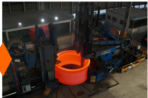
Ø11500 Ring Rolling Mill Upgrade
