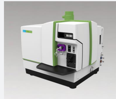
ICP-MS (Inductively Coupled Plasma- Mass Spectrometry) 금속불순물 분석장비
